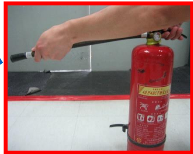
6: 喷嘴对准火源根部摇动喷嘴扫射
